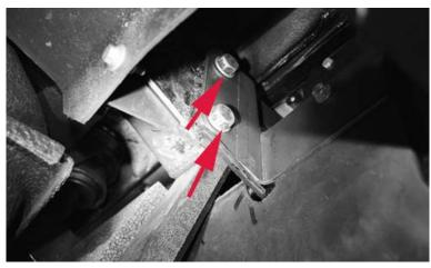
Position the mud flaps inside the bumper bracket, and reinstall the bolts.
