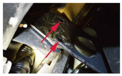
Start to work from one side, and do not release bolts from both sides of the bumper to prevent bumper misalignment.
