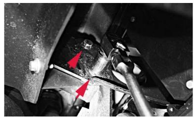
To mount the Mercedes G-Class rear mud flaps, you have to use the existing bumper to body bracket bolts.
