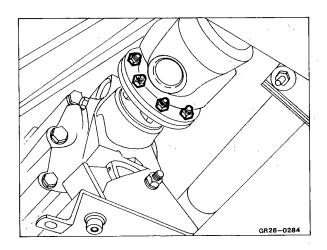
Note: In model 463, with homokinetic propeller shaft, the green color marking on the propeller shaft flange must be pointing right up and the vellow color marking on the component flange pointing right down.
