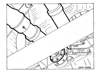
2 Turn arrow marking on the propeller shaft (slip joint area) right up.
