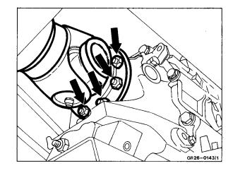
**Note:** In model 463, from 3.92 with homokinetic propeller shaft between transmission and transfer case, the mounting must be released from the transfer case.
