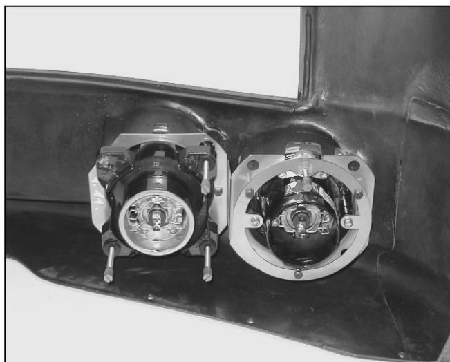
Figure 4 (Fitting of fog lamp)
